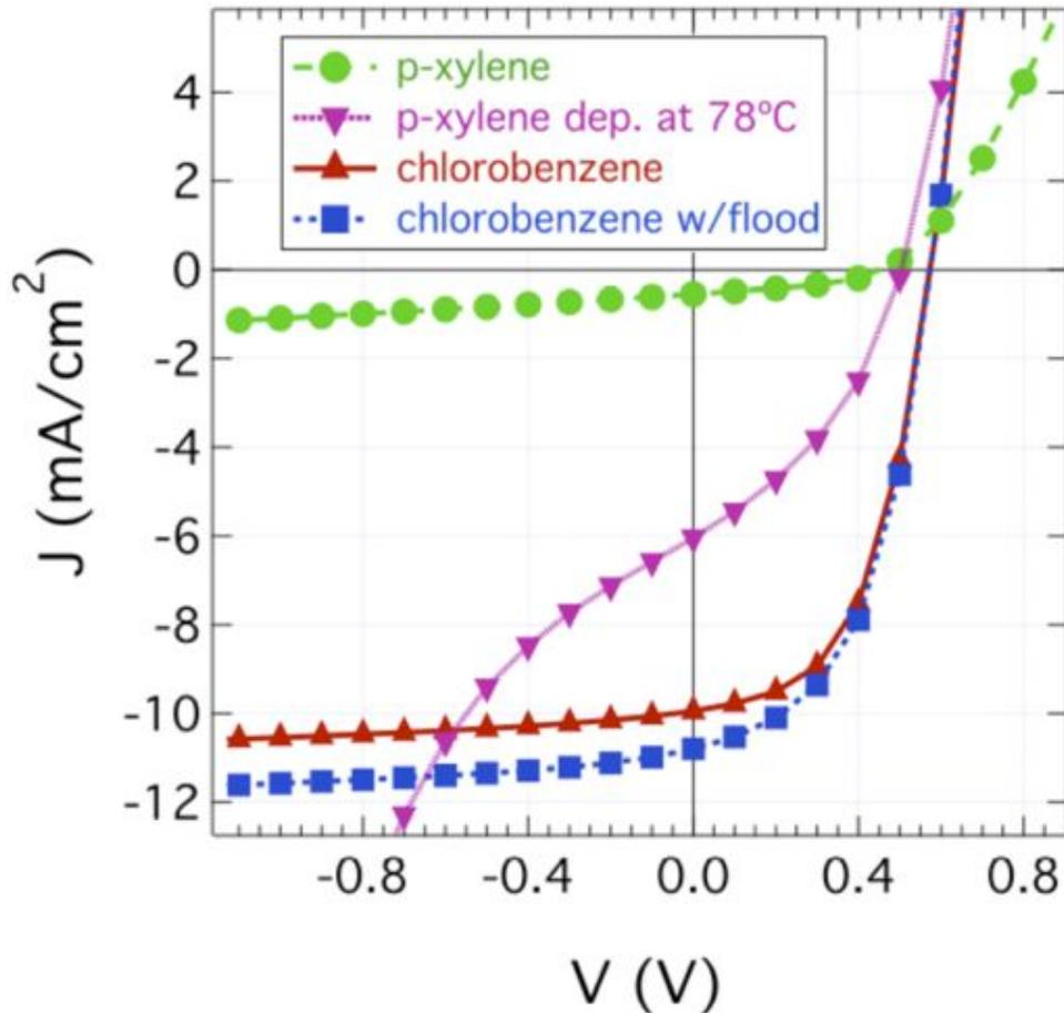
**Figure 3.** Measured illuminated (AM1.5 standard, i.e., at an air mass of 1.5) current density versus voltage curves for chlorobenzene-sprayed devices with and without an additional flood layer and p-xylene-sprayed devices at room temperature (25°C) and 78°C.
