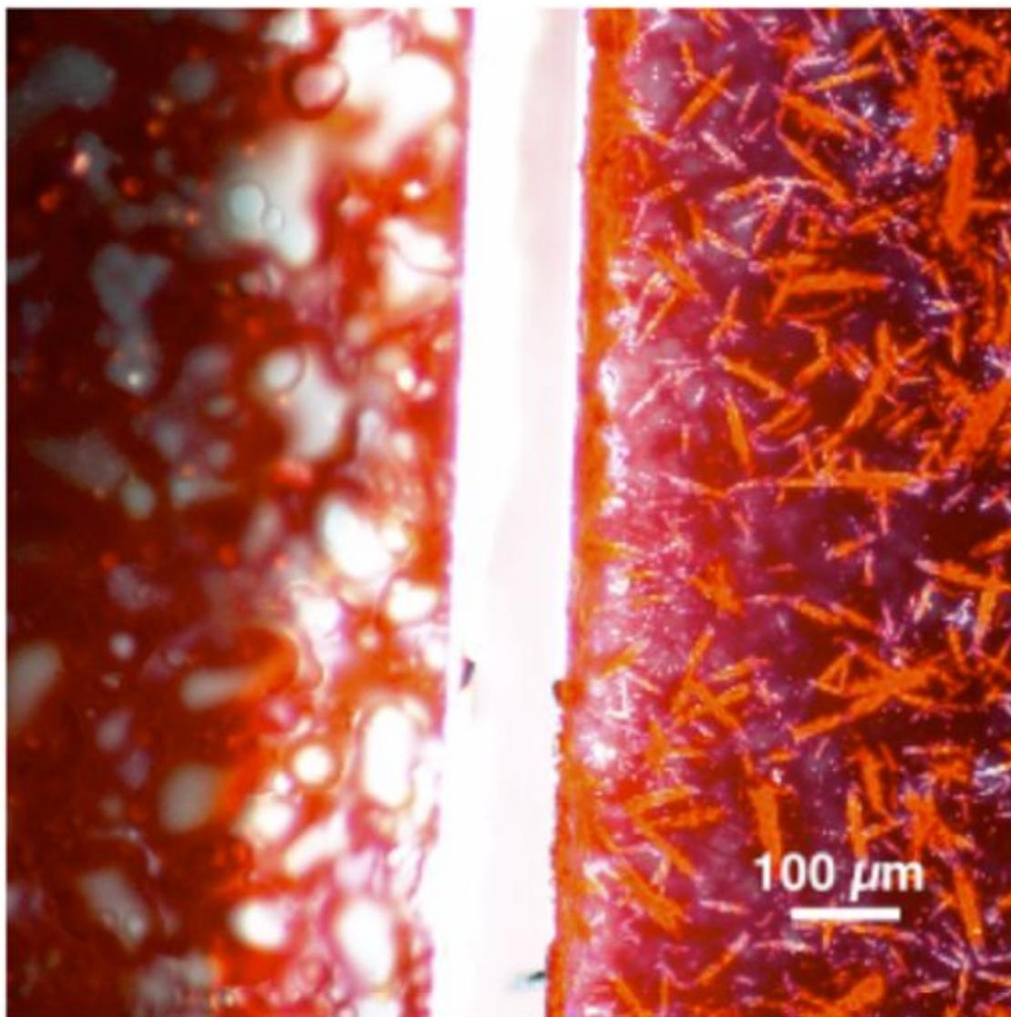
**Figure 2.** Dark-field optical micrograph of two separately deposited bulk-heterojunction P3HT:PCBM films sprayed using chlorobenzene (left) and p-xylene (right) as solvents.
