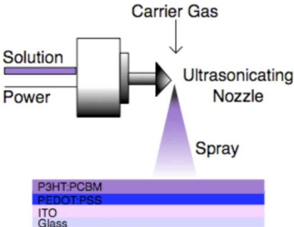
**Figure 1.** Ultrasonic spray deposition. Solution is delivered to the ultrasonic nozzle, creating a spray with uniform-diameter droplets. The spray is focused onto the substrate using nitrogen as the carrier gas. Thick films for this study were built up layer by layer. P3HT:PCBM: Poly(3-hexylthiophene):[6,6]phenyl-C61 butyric-methyl ester. PEDOT:PSS: poly(3,4-ethylenedioxythiophene):polystyrene sulfonate. ITO: Indium-tin oxide.
